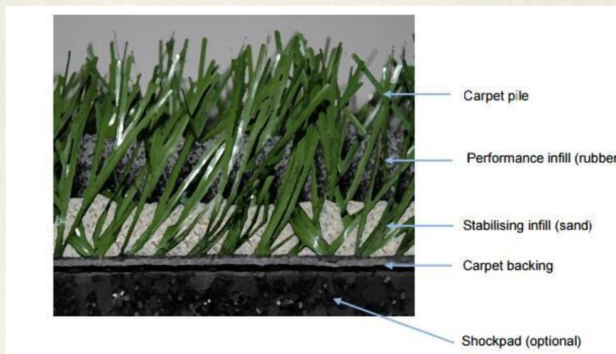
Figure 1. Schematic representation of an artificial turf system (Source: AVG, n/d).
